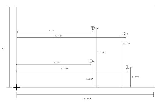
Main Controller Bare Board - P13321-PCB-MPCBA
