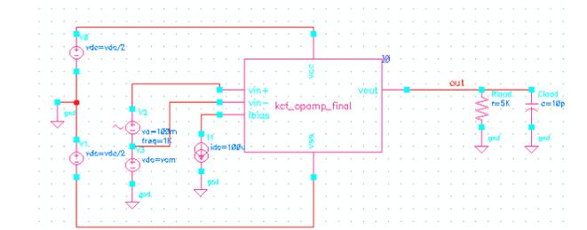
Figure 12. Open Loop Test Bench
