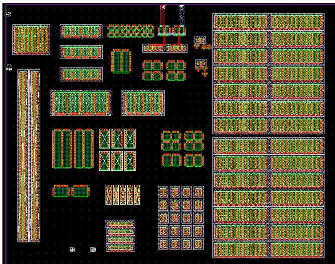
Figure 16. Physical Layout Floorplan
