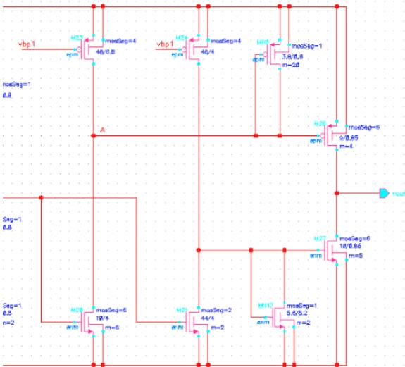
Figure 3. Common Source Level-Shift and Output Stage
