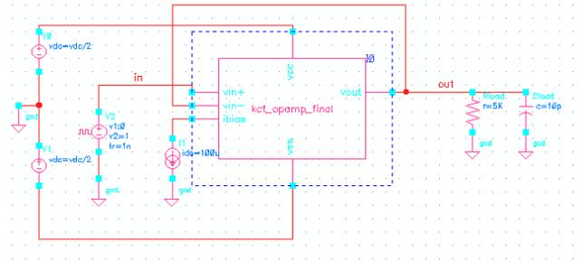
Figure 9. Slew Rate Test Bench
