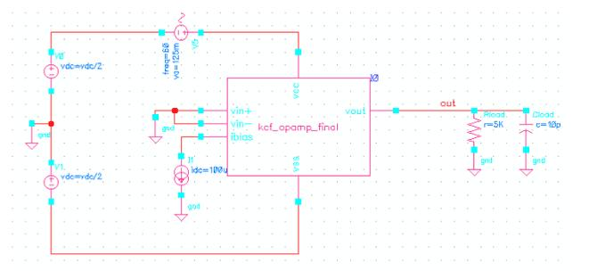
Figure 15. PSRR Test Bench
