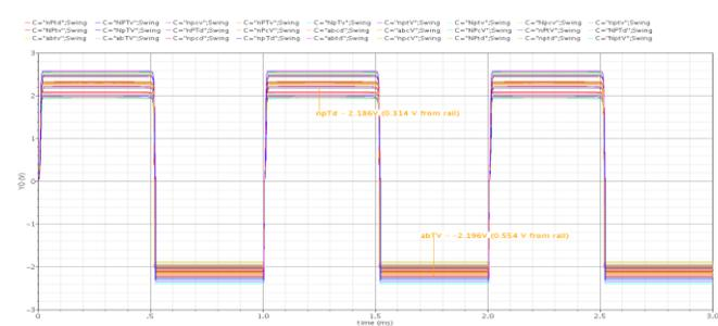
Figure 10. Large Signal Voltage Swing over Corners
