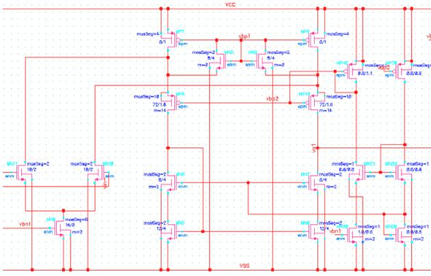
Figure 2. Folded Cascode stage with DC bias network
